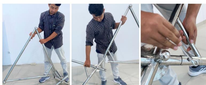
Figure 7. Illustration of assembling the robot's left and right legs on the stem
